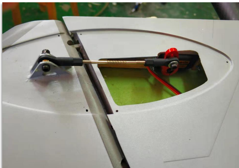
Flap servo mounting Control linkages : 50mm
